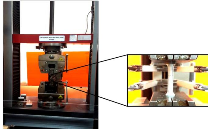
Figure 3. Universal testing machine.
