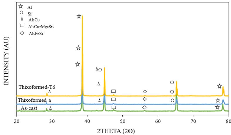
Figure 8. XRD pattern of as-cast, thixoformed and thixoformed-T6 Al-5.7Si-2Cu-0.3Mg.
